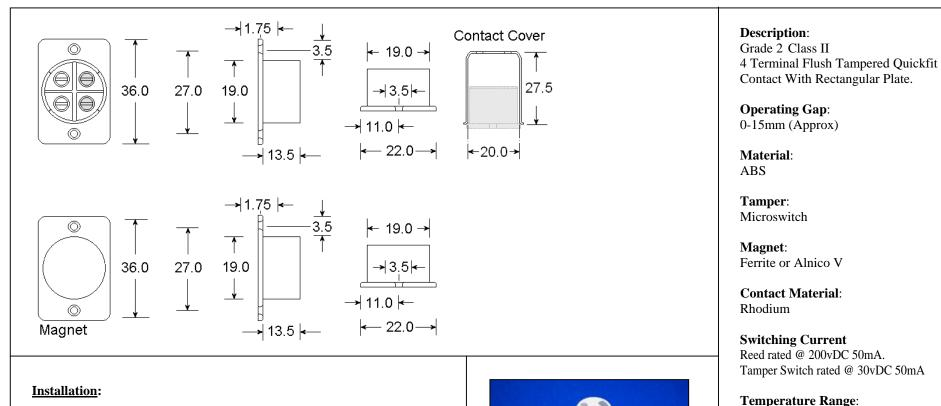
Connect the REED wires to the NICKEL terminals.
